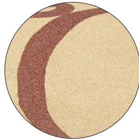
[P05] WET POUR 20mm Playtop Coloured Top Layer, 100mm Playtop Base Layer on 100mm compacted basecourse
