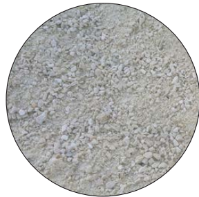
[P04] HOGGIN Permeable hoggins/self binding gravel paving to perimeter path. 70mm on 100mm compacted basecourse
